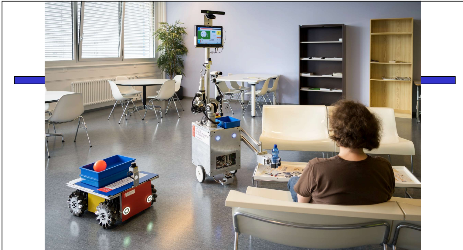
Figure 3. Original RH-Y and OP-Y robots, many times engaged in Robocup@Home competitions, shown here in a domestic task. The system is modular, featuring various configurations, all driven in Piaget environment
