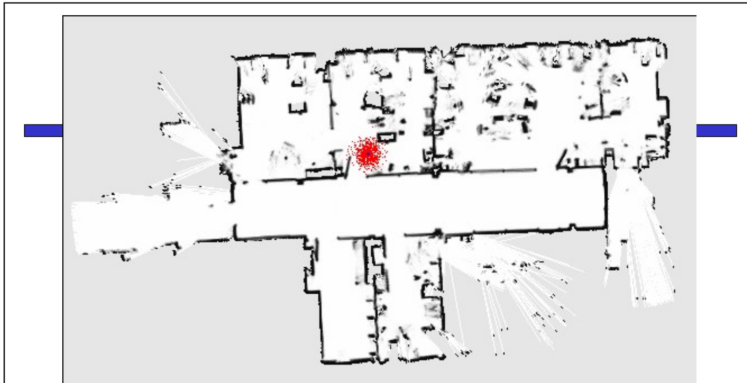
Figure 5. Example of a 2D map created using LiDAR data. The red blob represents the region where a robot is currently located in the map (ref. agv-iit-kgp.github.io , IIT Kharagpur, in [Madan and Gauthey, 2017]).
